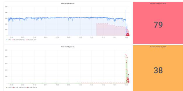
Fig. 5. Example of a Grafana dashboard to visualize the `netspot` output
